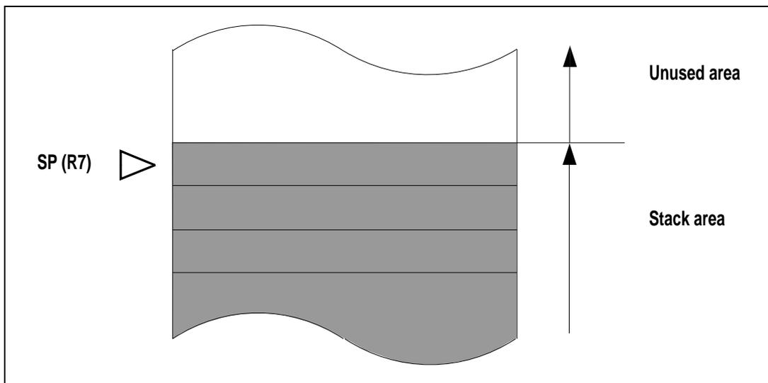
Figure 1-4. Stack Pointer
